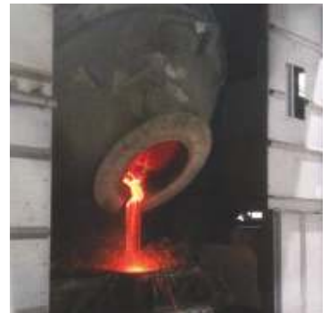
Slag tapping from front port by tilting
